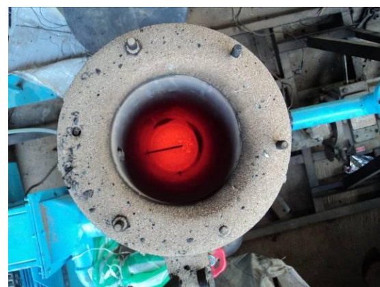
Fig 9: an aerial view of the BFBC during one of the experimental runs. Elutriated particles could be seen on top of the flange of the lower section. Inert bed temperature at this point is 801°C thus the red color of the inert bed, the dark straight line on top of the bed is the third thermocouple (temp. 627°C). This is made possible as a result of partitioning of the combustor body into lower section and upper section.
