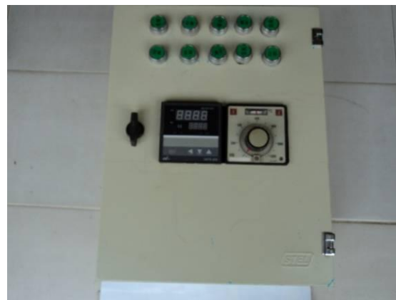
Fig.6: (a) Microscopy of the sand used as inert bed (b) A view of inside of the BFBC, (c) shows the control panel with 2 temperature controller and 10 normally-off push button (1 inactive).
